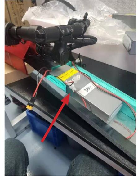
4. Remove the old battery and place new battery on the metal divider with the yellow connector sticking out through the cutout on the divider just like the old battery. Try to use the existing packaging foam to secure the new battery inside the metal divider so the battery does not move.
