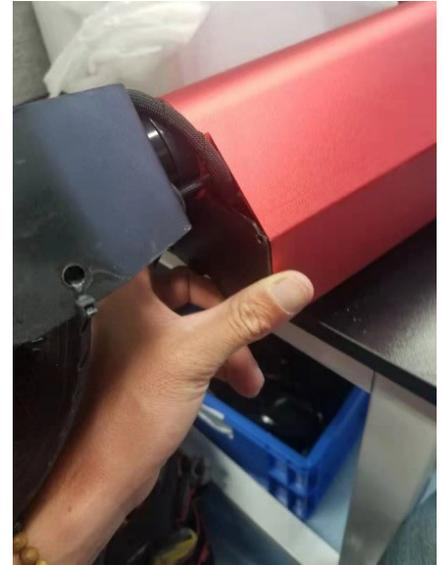
6. Once you are able to get the divider and all electronics back in the EZ-Ride, secure the bottom plate with the 4 screws from Step 1 using a 2.5mm hex key. Reattach the fender and light using the 4mm hex key if it was taken off. Then secure the top plate of the EZ-Ride.
